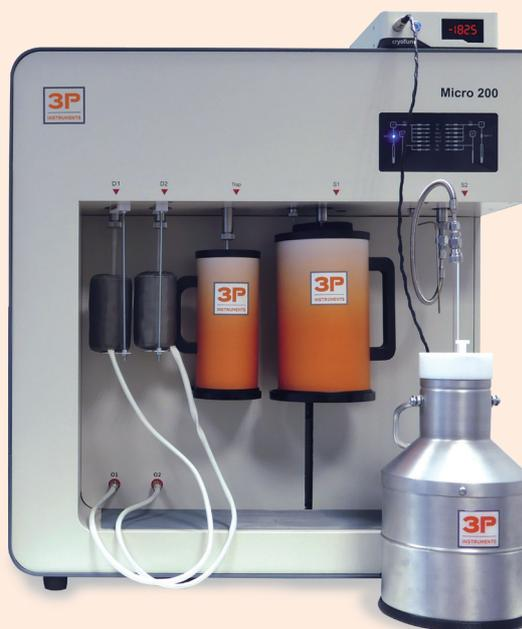
**Figure 9** The use of a cryoTune in connection with a 3P micro 200 instrument. The cryoTune is placed in the Dewar on the right and the small controller is positioned on the top of the instrument, the sample cell is connected with the measuring port.
