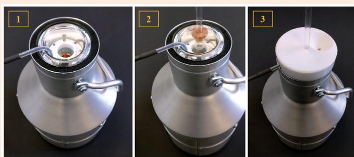
**Figure 8** The use of a cryoTune: the cryoTune is placed inside the Dewar (1). The sample cell is then placed into the cryoTune (2). Finally, the Dewar is closed with the special isolation cover (3). The little hole in the cover on the right enables refilling of liquid nitrogen during a long-term measurement (normally not necessary). The hole is covered during the measurement to optimize the Dewar holding time.
