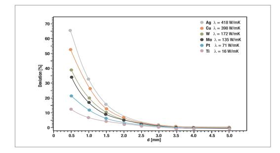
The graph from Schoderböck et. al., Int. J. Thermophys. (2009) illustrates the limitation of the classic Laserflash technique. Samples with a thickness of less than 2mm (depending on the thermal diffusivity of the material) already show a significant deviation from literature values.
